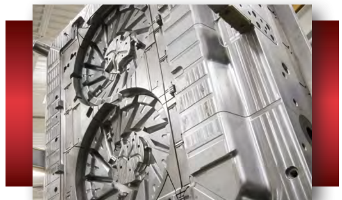
Tight-tolerance automotive molds like this are Cavalier’s fastest growing segment
